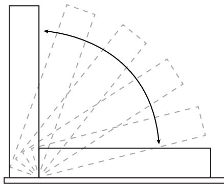
**EN** extremely easy to install and move thanks to fork slots in the bottom frame and a pivoting column
